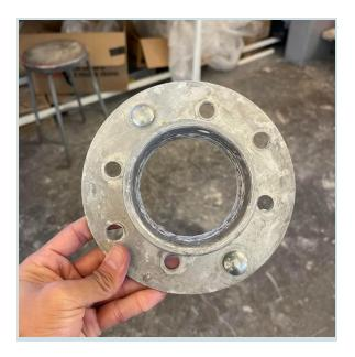
• With the tube adapter installed, you may now attach a clean tube to the adapter using the metal dowels.
