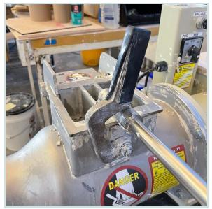
The locking arm should be closed before mixing or pugging. It may not fit completely over the arm, but the pugmill will operate as long as the chamber remains closed
