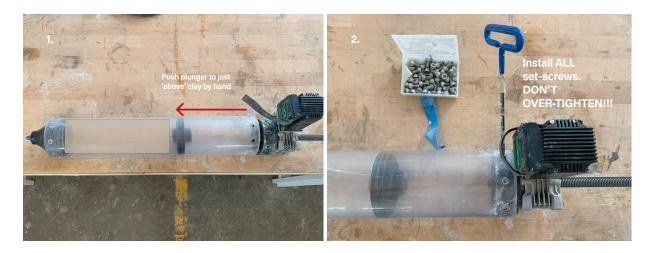
• Next, you will attach the extruder motor, which will start by inserting the ACME screw into the tube to align with the pocket at the top of the piston. If the tube is full of clay, it is very
