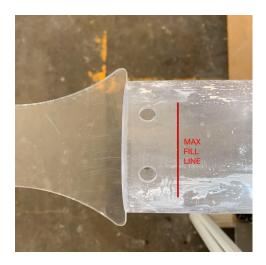
• Once the tube is full of clay per the limit indicated above, remove it from the pugmill by loosening the attachment hardware. Use the side labeled A (or "NOZZLE")) on the measuring stick and carve out excess clay from the side of the tube that was closest to the pugmill. This will be the nozzle side of the tube.
